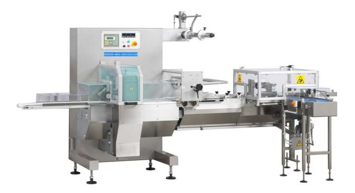
This automatic wrapping machine is specially designed for the use with dry ice slices and / or blocks. All parts in contact with the product are made of stainless steel. Automatic pitch change on conveyor and all motors are torque controlled. The temperature for welding is shown on the display and is electronically controlled. The control panel consists of various instruments and visual alarms and is equipped with a self-diagnostic device.
